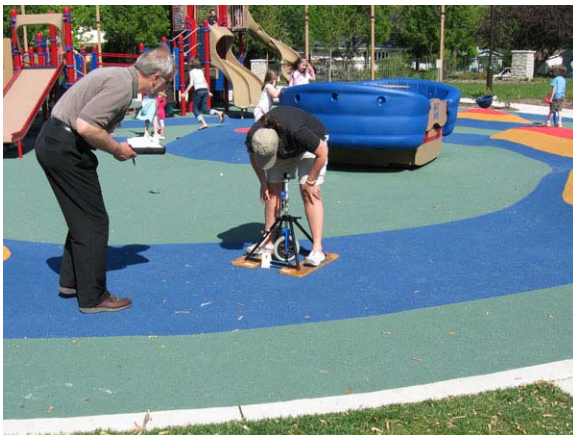
Photo 3: PIP location measured for firmness and stability using Rotational Penetrometer.
