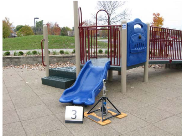
Photo 6: TIL at egress for slide.
