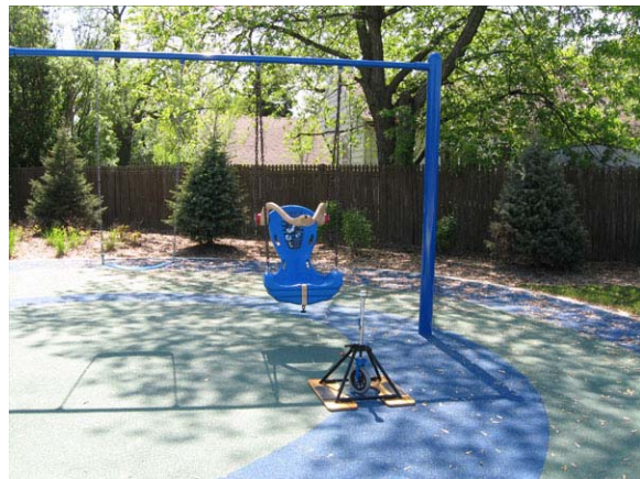
Photo 4: PIP location at swings found in non-compliance with HIC scores over 1,000.
