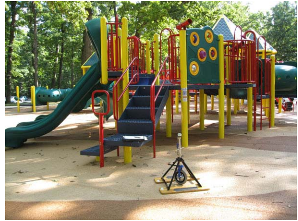
Photo 14: HYB surface system with rubber mat top layer over shredded rubber base contained in pillow forms.
